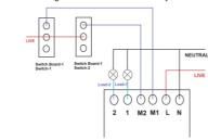
2-Way SMART SWITCH PRODUCT SHOULD INSTALL AT SWITCH BOARD-2 WHERE THE LOADS ARE CONNECTED
